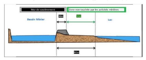
The "berm" diagram from the SEMP presents a 30metre dam against the dredge pond, and a 50 m buffer between the dam and the lake. The actual distances are not correct as explored in the article.
